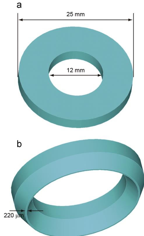
Fig. 2. Ceramic dimensions of the (a) stator and (b) rotor sides.
