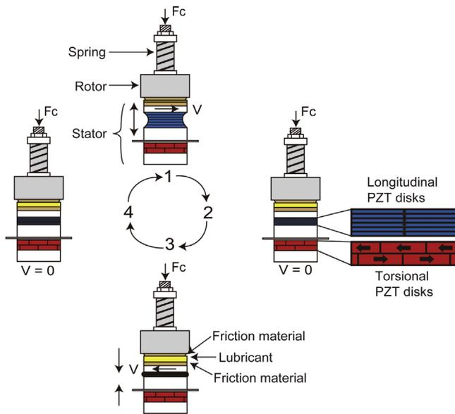
Fig. 1. Principle of operation for a hybrid transducer-type ultrasonic motor.
