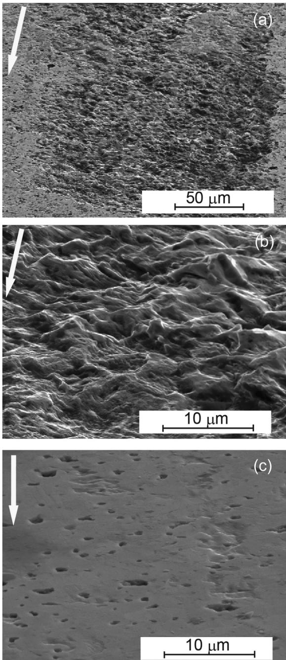
**Fig. 8.** (a) Scanning electron micrograph of the worn SiC surface with both fractured and smooth morphologies on the rotor side. Magnified views of the area inside the (b) fractured region and (c) smooth region. The sample tilt was equal to 70°. The arrows indicate the sliding directions.
