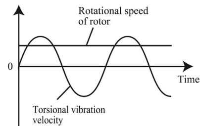
Fig. 4. Graph illustrating the change in sliding velocity of an ultrasonic motor.
