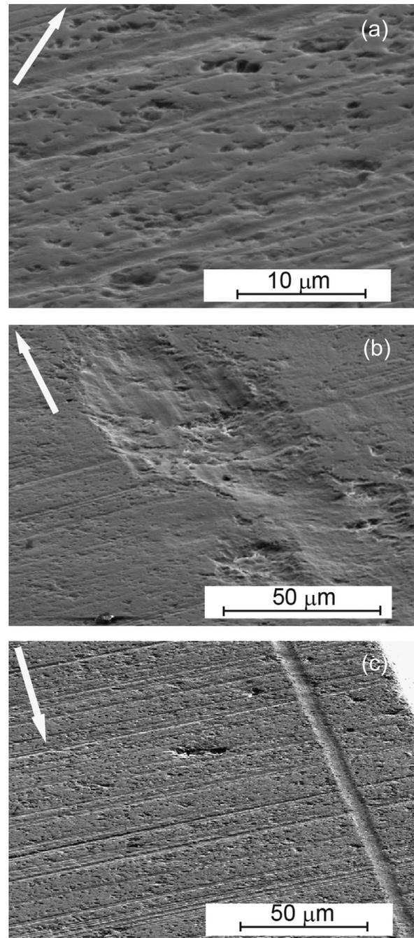
**Fig. 9.** Scanning electron micrographs of the worn  $\text{Si}_3\text{N}_4$  surface: (a) mild wear region; (b) region with a groove on the stator side; (c) region with a groove on the rotor side. The sample tilt was equal to 70°. The arrows indicate the sliding directions.
