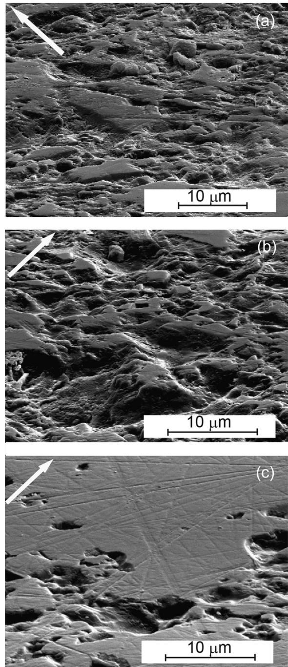
Fig. 5. (a) Scanning electron micrograph of the worn  $\text{Al}_2\text{O}_3$  surface on the rotor side. Scanning electron micrographs showing (b) the fractured region and (c) the mild wear region on the worn  $\text{Al}_2\text{O}_3$  surface on the stator side. The sample tilt was equal to 70°. The arrows indicate the sliding directions.
