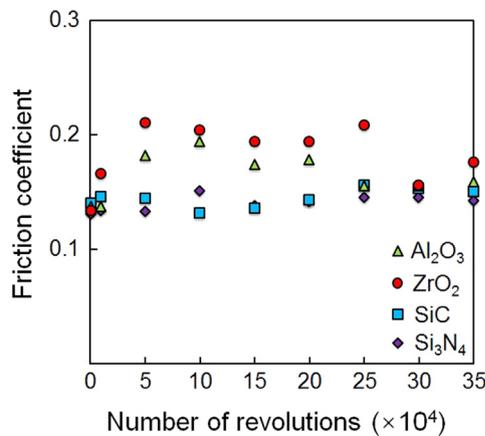
Fig. 10. Measured dependence of the friction coefficient on the number of revolutions for various ceramic materials.
