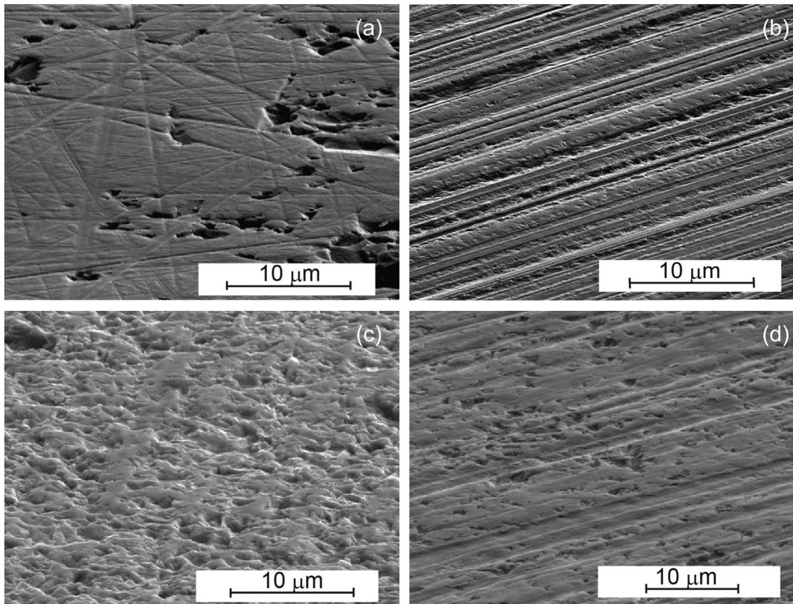
Fig. 3. Scanning electron micrographs of the unworn surfaces of the (a)  $\text{Al}_2\text{O}_3$ , (b)  $\text{ZrO}_2$ , (c)  $\text{SiC}$ , and (d)  $\text{Si}_3\text{N}_4$  ceramics. The sample tilt was equal to  $70^\circ$ .
