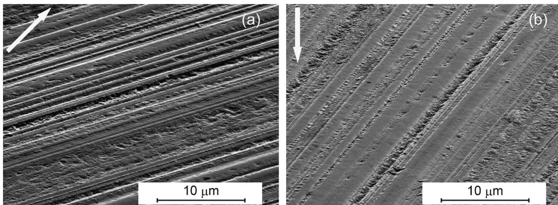
**Fig. 7.** Scanning electron micrographs of the worn  $\text{ZrO}_2$  surface on the (a) stator side and (b) rotor side. The sample tilt was equal to  $70^\circ$ . The arrows indicate the sliding directions.
