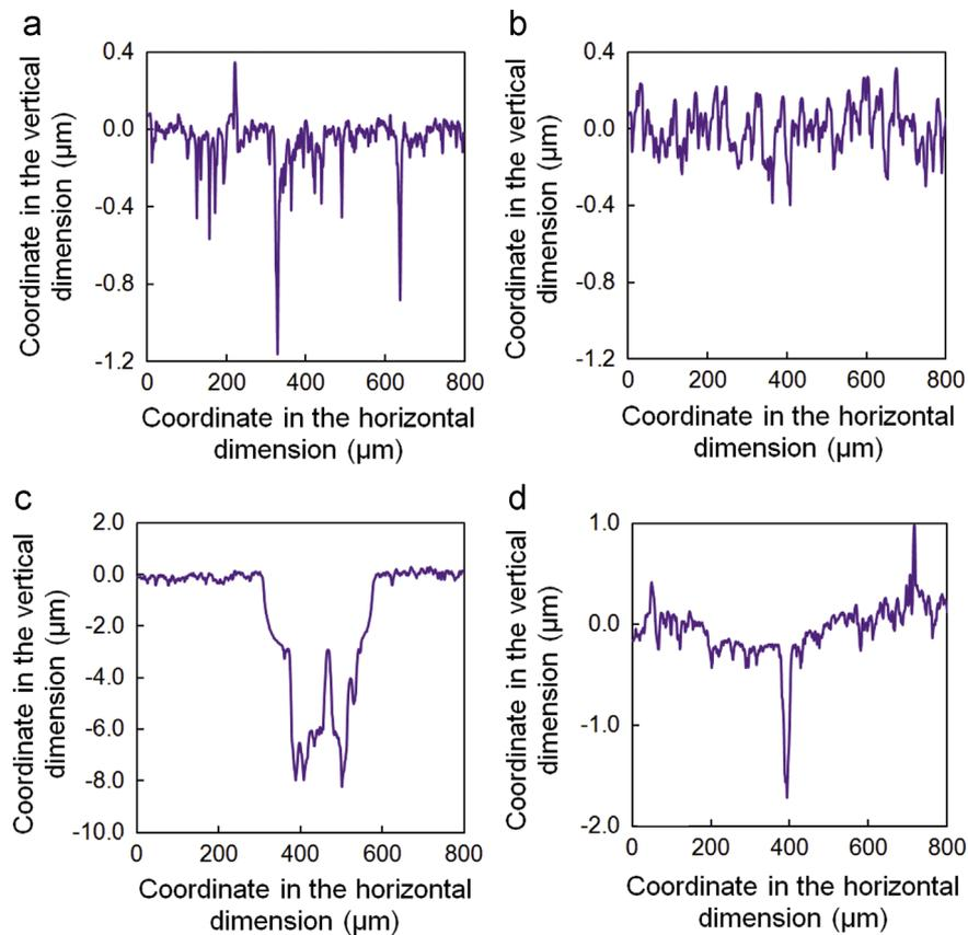
**Fig. 6.** Worn surface profiles of the (a)  $\text{Al}_2\text{O}_3$ , (b)  $\text{ZrO}_2$ , (c)  $\text{SiC}$  (fractured region), and (d)  $\text{Si}_3\text{N}_4$  (polished region) ceramics on the stator side.
