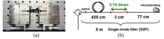
Fig. 2. (a) FUT prepared by fixing an SMF on the translation stage with epoxy glue. (b) Schematic of the structure of the FUT.
