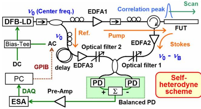
Fig. 1. Experimental setup of the BOCDR system. AC: alternating current; DAQ: data acquisition; DC: direct current; DFB-LD: distributed-feedback LD; GPIB: general-purpose interface bus; PC: personal computer; PD: photodiode.
