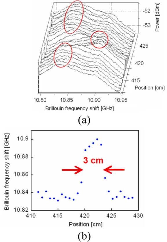
Fig. 3. (a) Distribution of the BGS along the FUT. (b) Distribution of the BFS along the FUT. Spatial resolution better than  $3 \text{ cm}$  was achieved with  $0.02 \text{ s/point}$  sampling rate. A resolution of one-half ( $15 \text{ mm}$ ) of the marked width is obviously available.
