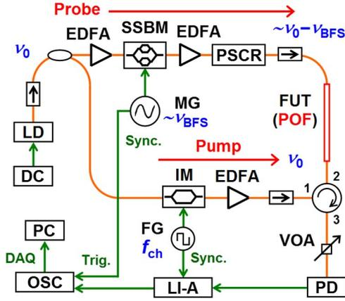
Fig. 1. (Color online) Experimental setup for observing SBS in POF with pump-probe technique. DAQ, data acquisition; DC, direct current; LD, laser diode; EDFA, erbium-doped fiber amplifier; FG, function generator; FUT, fiber under test; IM, intensity modulator; LI-A, lock-in amplifier; MG, microwave generator; OSC, oscilloscope; PC, personal computer; PD, photodetector; POF, polymer optical fiber; PSCR, polarization scrambler; SSBM, single-sideband modulator; VOA, variable optical attenuator.
