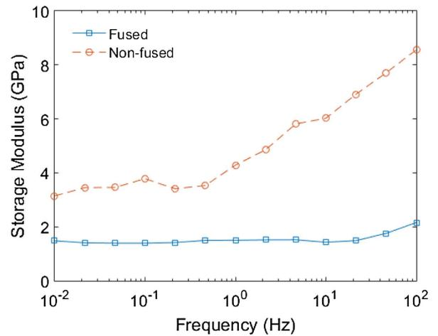
**Fig. 3.** Frequency response of fused and non-fused POFs.
