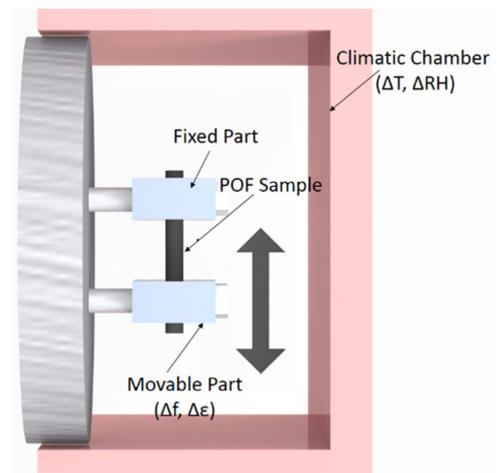
Fig. 1. Experimental setup employed for the DMA on the POFs.
