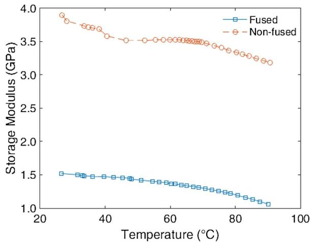
**Fig. 2.** Temperature response of fused and non-fused POFs.
