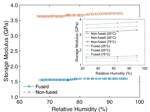
**Fig. 4.** Storage modulus as a function of RH of about 30% (from 66% to 96%) for the fused and non-fused POFs. The inset shows the storage modulus as a function of the RH at three different temperatures.
