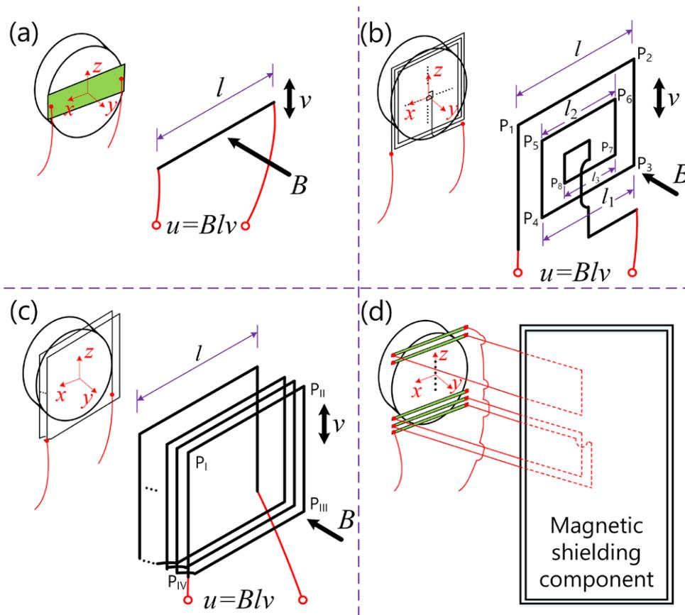
Figure 2. Output voltage induced by (a) a metal plate or wire, (b) a rectangular spiral coil, (c) a rectangular helix coil, and (d) parallel coils connected with magnetic-shielded leads.
