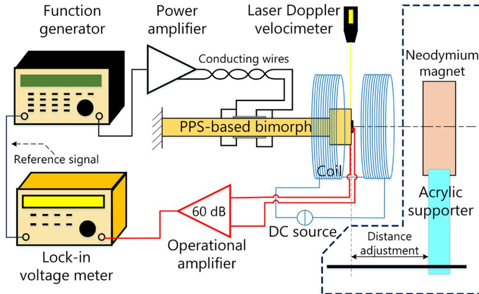
Figure 3. Experimental setup for measuring the magnetic field.
