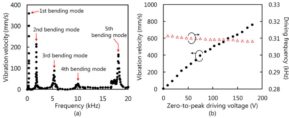
Figure 4. Vibration velocity as functions of (a) frequency at 60  $V_{0-p}$  and (b) driving voltage at approximately 0.31 kHz.
