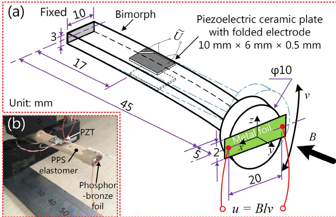
Figure 1. Magnetic field sensor with a PPS-based bimorph: (a) its schematic and dimensions and (b) a picture of the prototype.
