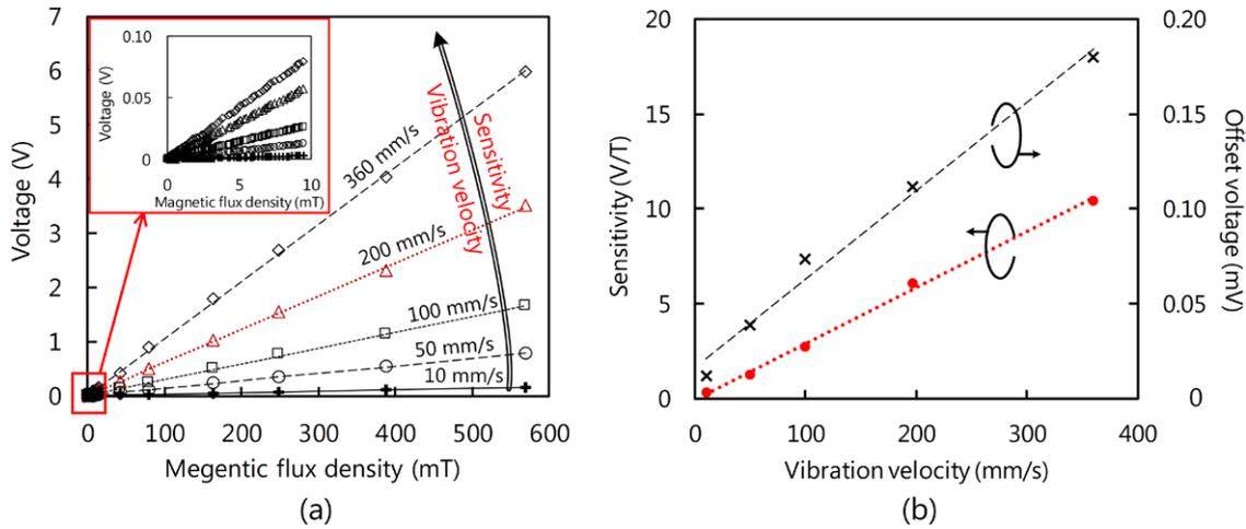
Figure 5. Experimental results: (a) output voltage versus magnetic flux density at vibration velocities of 10, 50, 100, 200, and 360  $\text{mm s}^{-1}$ , and (b) sensitivity and offset voltage as a function of vibration velocity.
