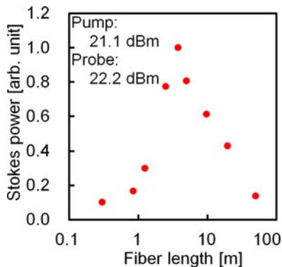
Fig. 4. Stokes power dependence on POF length.
