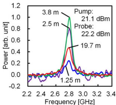
Fig. 3. Measured BGS dependence on POF length.
