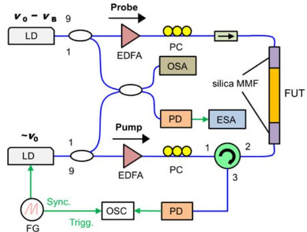
Fig. 1. Experimental setup for observing SBS in POF with pump-probe technique. EDFA, erbium-doped fiber amplifier; ESA, electrical spectrum analyzer; FG, function generator; FUT, fiber under test; LD, laser diode; OSA, optical spectrum analyzer; OSC, oscilloscope; PC, polarization controller; PD, photodetector.
