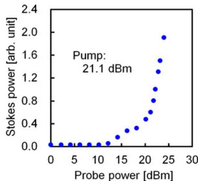
Fig. 6. Stokes power dependence on probe power.
