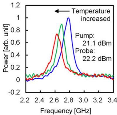
Fig. 8. Measured BGS dependence on temperature.
