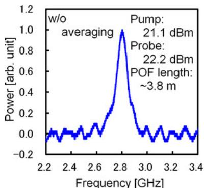
Fig. 2. Measured BGS in 3.8-m-long POF without averaging.
