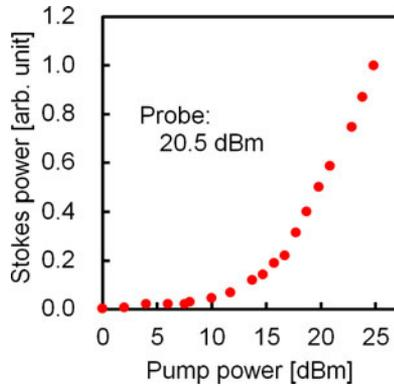
Fig. 7. Stokes power dependence on pump power.
