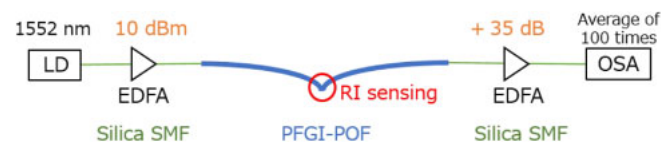
Fig. 2. (Color online) Schematic of the experimental setup for refractive index sensing. EDFA, erbium-doped fiber amplifier; LD, laser diode; OSA, optical spectrum analyzer.
