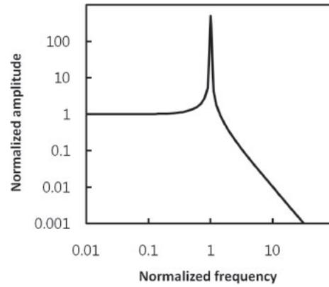
Fig. 2. Amplitude characteristics of an accelerometer.
