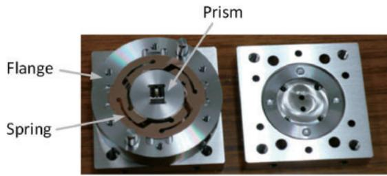
Fig. 3. (Color) Inside of the spring-suspended mass (with the outer flange removed).
