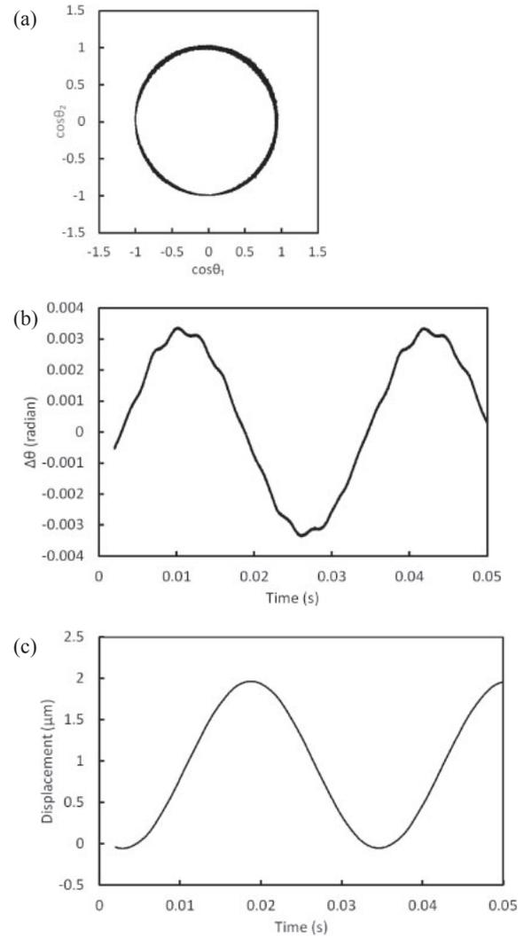
**Fig. 6.** (a) Lissajous figure for  $\cos \theta_1$  and  $\cos \theta_2$ . (b) Values of  $\Delta\theta$ . (c) Waveforms obtained by integrating (b).
