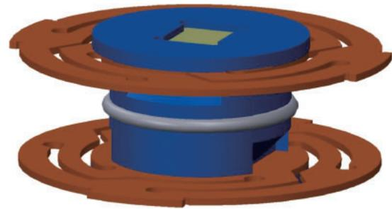
Fig. 4. (Color) 3D CAD model of the vibrating part in the sensor.
