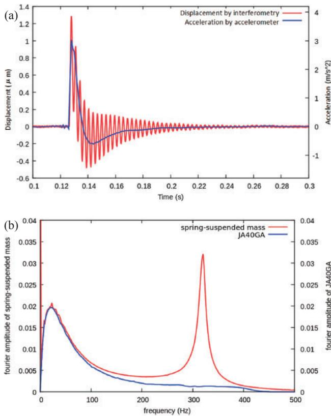
**Fig. 7.** (Color) (a) Acceleration measured using the accelerometer and displacement of the sensor obtained using light interferometry. (b) Fourier spectra of the accelerometer and spring-suspended mass.
