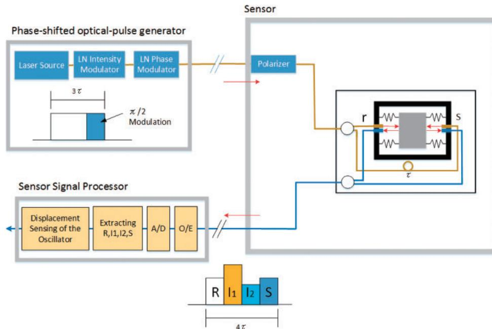
Fig. 5. (Color) Structure of the test bed in phase-shifted optical pulse interferometry. This method uses laser-pulse inputs  $R$  and  $S$ . The pulse duration is 30 ns. The phase of the last 10 ns is progressed (regressed) to  $\pi/2$  against the first 20 ns. This pulse is transmitted every 1  $\mu$ s.
