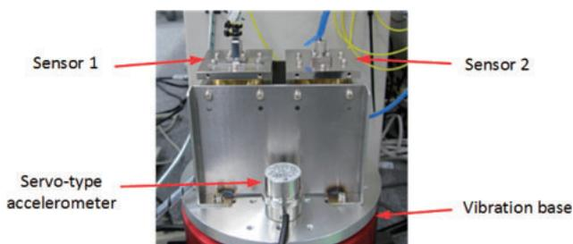
**Fig. 10.** (Color) Photograph of the spring-suspended mass and sensor during observations.
