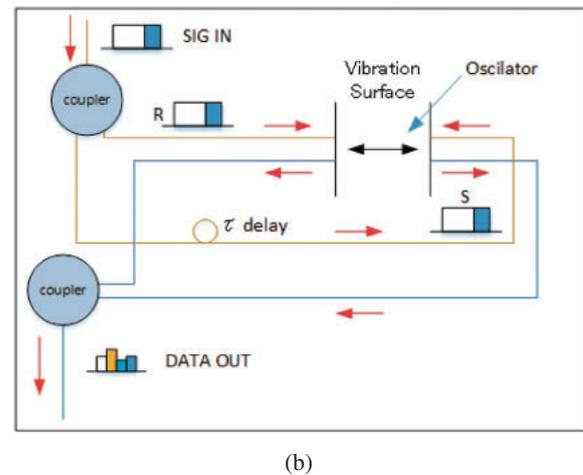
Fig. 1. (Color) (a) Schematic diagrams of reference light, measurement light, and interference light. (b) Schematic diagram of phase-shifted optical pulse interferometry.
