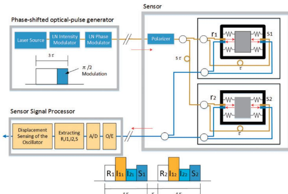
**Fig. 9.** (Color) Configuration diagram of the test bed when conducting simultaneous multiple observations with phase-shifted optical pulse interferometry. This method uses laser-pulse inputs  $R$  and  $S$ . The pulse duration is 30 ns. The phase of the last 10 ns is progressed (regressed) to  $\pi/2$  against the first 20 ns. This pulse is transmitted every  $1 \mu\text{s}$ .
