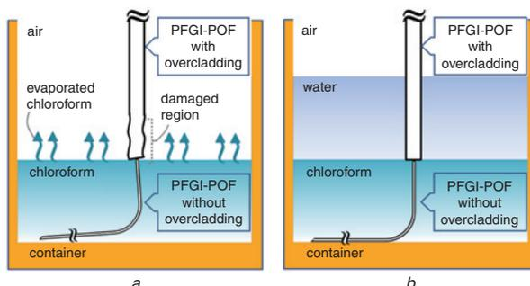
**Fig. 1** Schematic setups for etching overcladding layers of PFGI-POFs using chloroform only, and chloroform and water
