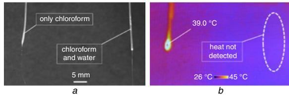
**Fig. 3** Photograph and infrared thermal image, of PFGI-POFs with overcladding layers etched using chloroform only (left), and chloroform and water (right)
