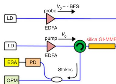
**Fig. 1** Experimental setup for observing SBS in silica GI-MMF with pump-probe technique
