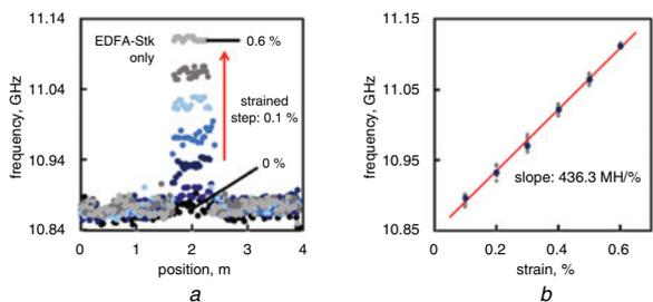
**Fig. 5** Results of distributed strain measurement (2)
