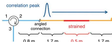
**Fig. 2** Structure of FUT for distributed measurement
