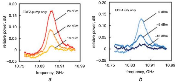
**Fig. 3** Dependence of the measured BGSs on the output power of the EDFAs
