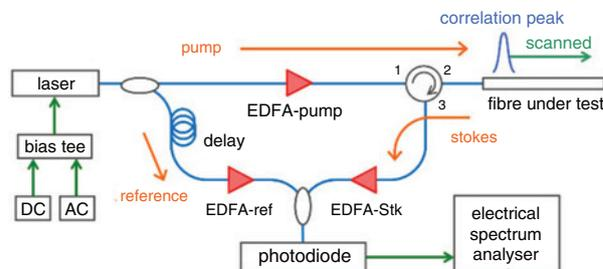
**Fig. 1** Schematic setup of conventional BOCDR involving three EDFAs. AC, alternating current; DC, direct current
