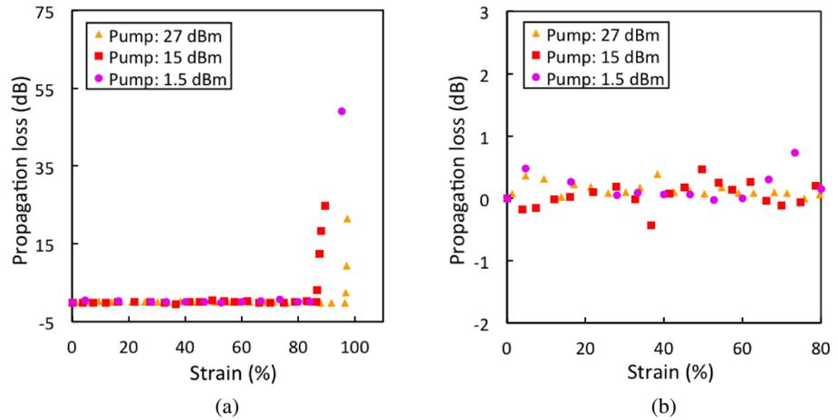
Fig. 2. (a) Propagation loss vs applied strain at three different optical powers, and (b) a magnified view of the strain from 0 to 80%.
