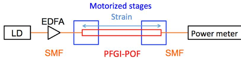
**Fig. 1.** Schematic of experimental setup. EDFA, erbium-doped fiber amplifier; LD, laser diode; PFGI-POF, perfluorinated graded-index plastic optical fiber; SMF, single-mode fiber.
