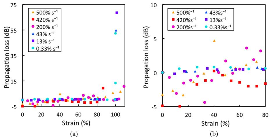
Fig. 3. (a) Propagation loss vs applied strain at six different strain rates, and (b) its magnified view in the strain range below 80%.
