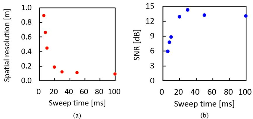
Fig. 4. Measured sweep-time dependences of (a) the spatial resolution and (b) the signal-to-noise ratio (SNR).
