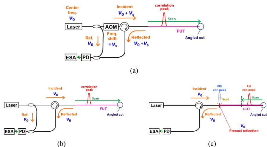
**Fig. 1.** Schematic experimental setups of (a) standard optical correlation-domain reflectometry (OCDR) [15], (b) acousto-optic modulator (AOM)-free OCDR [21], and (c) further simplified AOM-free OCDR using a polymer optical fiber (POF). ESA, electrical spectrum analyzer; FUT, fiber under test; PD, photo detector.
