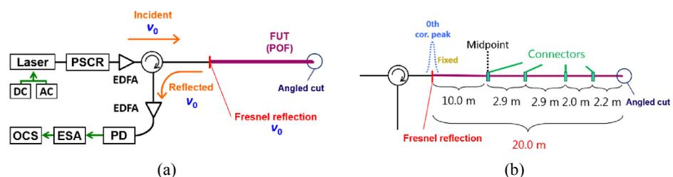
Fig. 2. (a) Actual experimental setup of further simplified AOM-free OCDR using a POF, and (b) the structure of the fiber under test (FUT). AC, alternating current; DC, direct current; EDFA, erbium-doped fiber amplifier; OSC, oscilloscope; PSCR, polarization scrambler.
