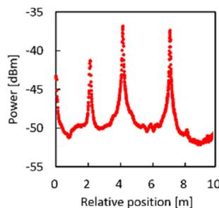
Fig. 3. Measured distribution of the Fresnel-reflected power.
