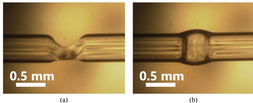
**Fig. 3.** Micrographs of the crushed polymer optical fiber: (a) side view and (b) top view.
