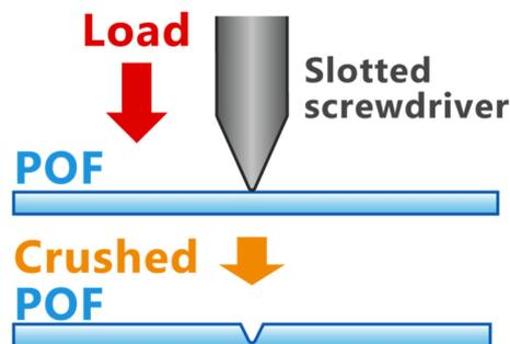
**Fig. 1.** Processing procedure of the crushed polymer optical fiber (POF).
