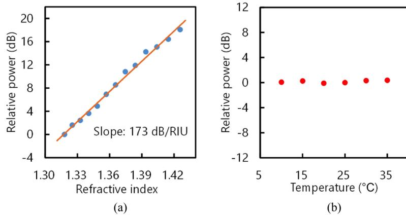
**Fig. 4.** (a) Measured relative transmitted power dependence on the refractive index (RI). (b) Relative transmitted power dependence on temperature when the refractive index was 1.366.
