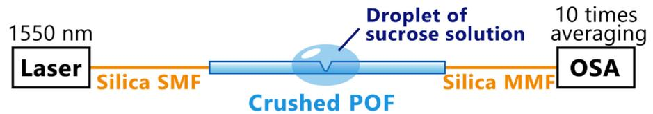
**Fig. 2.** Experimental setup for the refractive index sensing using the crushed polymer optical fiber (POF). MMF: multimode fiber, OSA: optical spectrum analyzer, and SMF: single-mode fiber.
