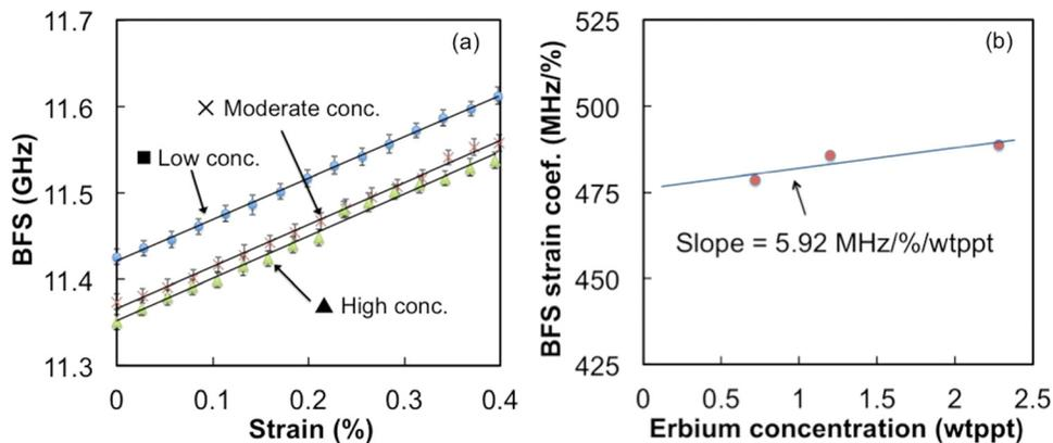
FIG. 5. (a) Measured BFS dependence on strain in EDFs with different erbium concentrations. (b) Strain coefficient of BFS in EDFs as a function of erbium concentration.
