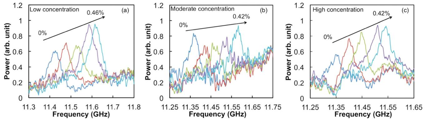
FIG. 4. Measured BGS dependences on strain in EDFs with erbium concentrations of (a) 0.72 wtppt (low), (b) 1.20 wtppt (moderate), and (c) 2.28 wtppt (high).
