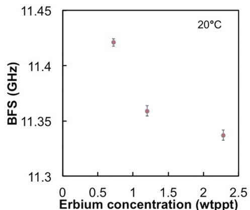
FIG. 2. BFS in EDFs at 20°C as a function of erbium concentration.
