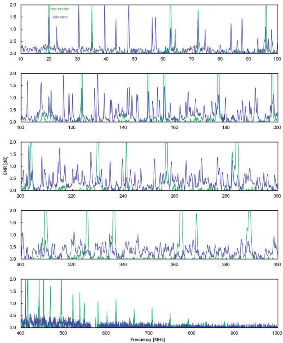
Fig. 3. Measured spontaneous depolarized GAWBS: spectra in side (blue) and center (green) cores.
