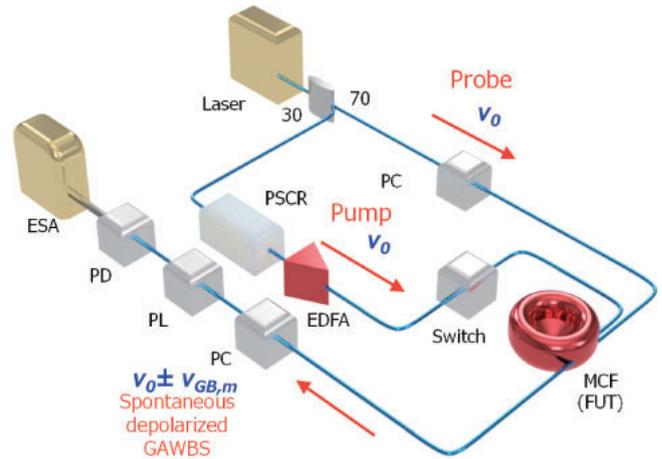
Fig. 2. Schematic setup for observing spontaneous depolarized GAWBS. EDFA, erbium-doped fiber amplifier; ESA, electrical spectrum analyzer; FUT, fiber under test; MCF, multicore fiber; PC, polarization controller; PD, photodetector; PL, polarizer; PSCR, polarization scrambler.
