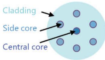
Fig. 1. Cross section of the multicore fiber under test.
