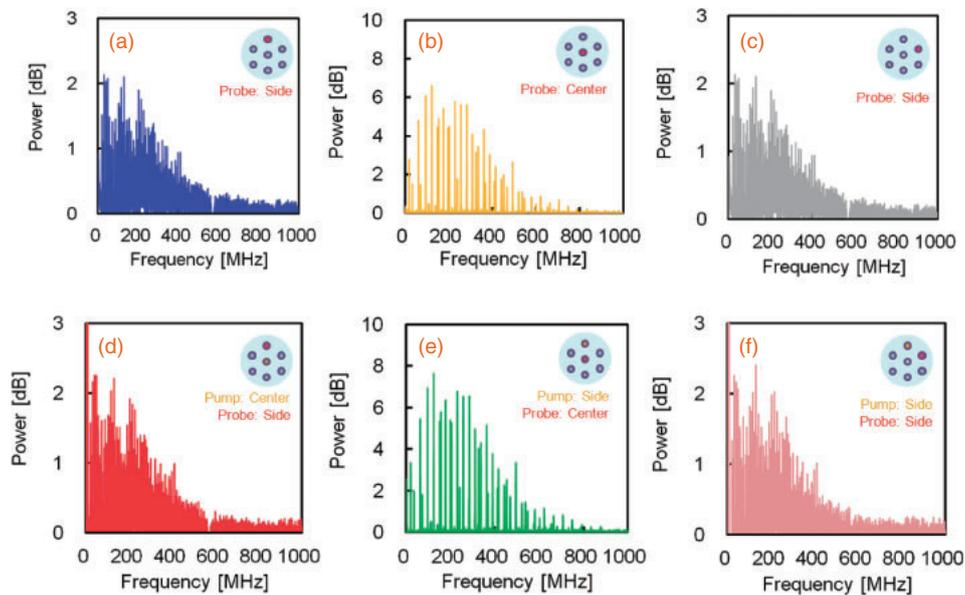
Fig. 4. Depolarized GAWBS spectra in the (a) side core, (b) central core, and (c) side core in the vicinity of the first. GAWBS spectra with the interaction between acoustic waves in the (d) side core and central core (pump light into the center core and probe light into the side core), (e) side core and central core (pump light into the side core and probe light into the central core), and (f) side core and another side core (in the vicinity).
