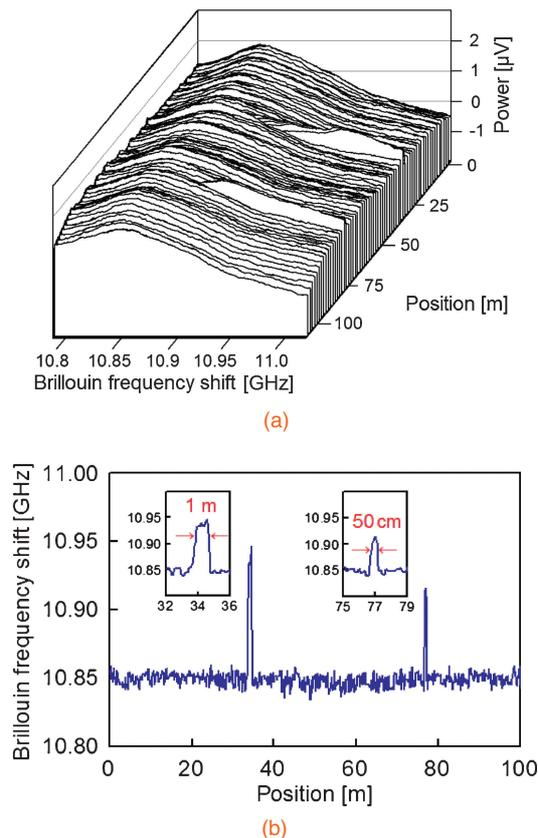
**Fig. 5.** Measured distributions of (a) BGS and (b) BFS. The insets in (b) show the magnified views around strain-applied positions.
