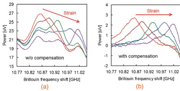
**Fig. 4.** Measured BGS (a) without and (b) with noise-floor compensation. Strains of 0, 0.08, 0.16, 0.24, and 0.32% were applied.
