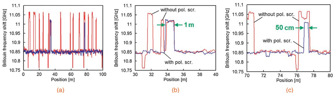
**Fig. 3.** (a) Measured distribution of the Brillouin frequency shift (BFS) along the entire length of the 100-m FUT with (blue) and without (red) a polarization scrambling, (b) its magnified view with the range of 30–40 m, and (c) that with the range of 70–80 m.
