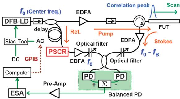
**Fig. 1.** Experimental setup of BOCDR with polarization scrambling: AC, alternating current; DC, direct current; DFB-LD, distributed-feedback laser diode; EDFA, erbium-doped fiber amplifier; ESA, electrical spectrum analyzer; FUT, fiber under test; GPIB, general-purpose interface bus; PD, photo-diode; PSCR, polarization scrambler.
