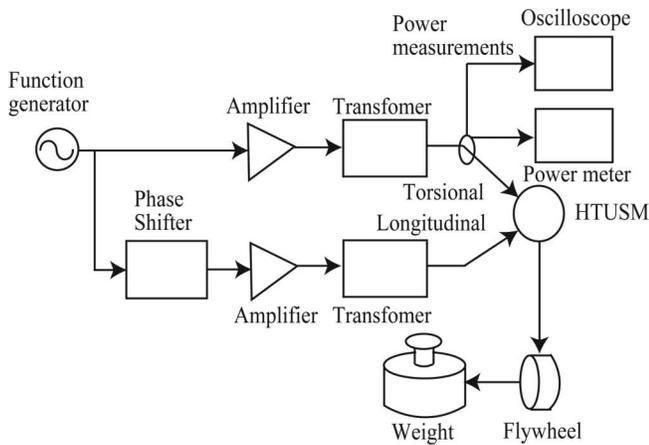
Fig. 13. Diagram of experimental setup.
