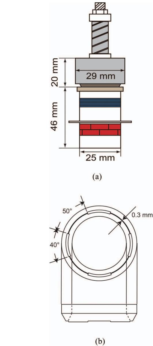
Fig. 12. (a) Dimension of the hybrid transducer-type ultrasonic motor used in the experiment and (b) design of the contact side of the rotor.
