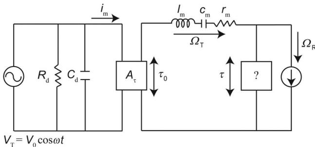
Fig. 4. Equivalent circuit of the hybrid transducer-type ultrasonic motor for torque transmission mechanism.
