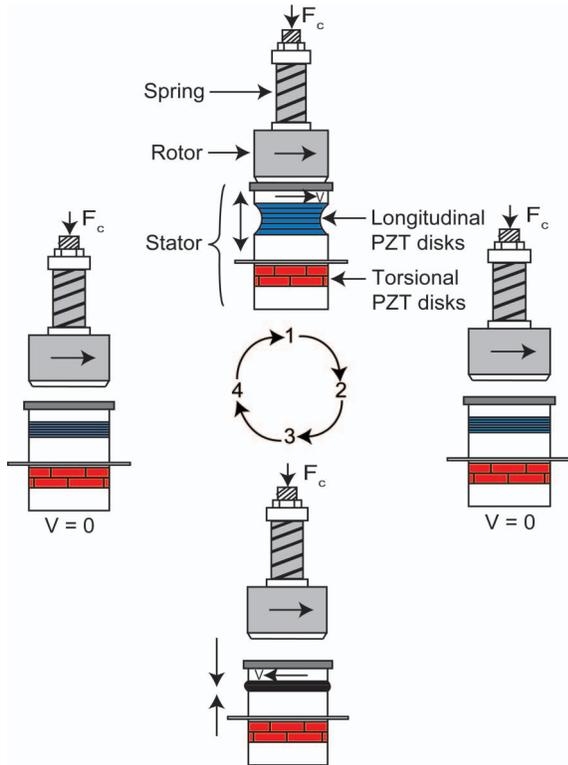
Fig. 1. Operating principle of the hybrid transducer-type ultrasonic motor.
