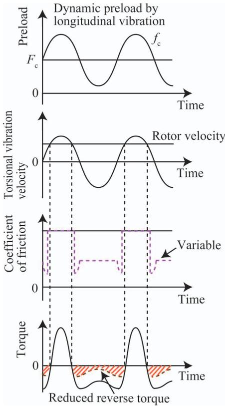
Fig. 3. Lubrication mechanism in the hybrid transducer-type ultrasonic motor.
