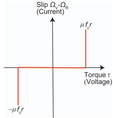
Fig. 5. Coulomb friction model used in calculation for the dry condition.
