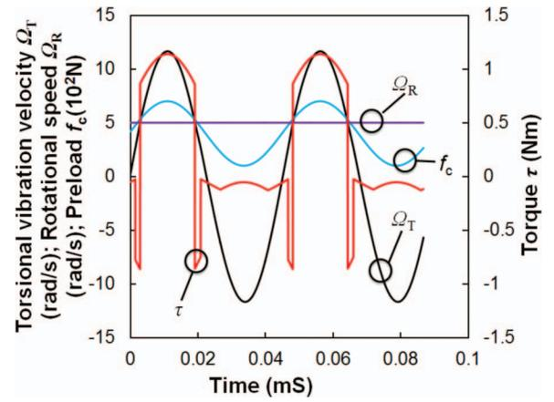
Fig. 8. Instantaneous waveforms of torsional vibration velocity  $\Omega_T$ , rotational speed  $\Omega_R$ , torque  $\tau$ , and dynamic preload  $f_c$ .
