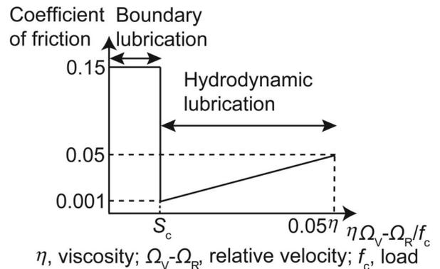
Fig. 6. Stribeck curve used in calculation for the lubricated condition.
