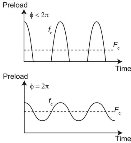
Fig. 7. Waveforms of dynamic preload.
