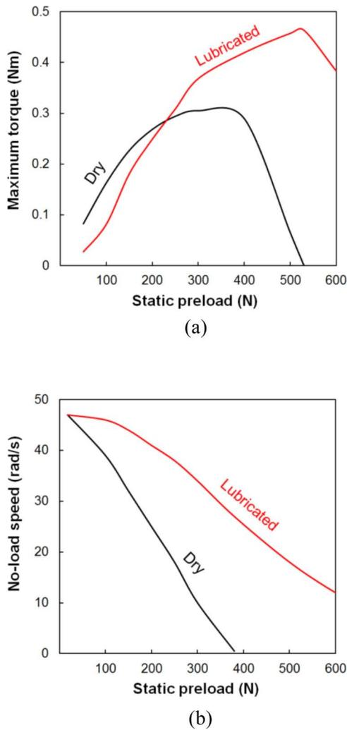
Fig. 11. Calculated dependences of (a) maximum torque and (b) no-load speed on static preload.
