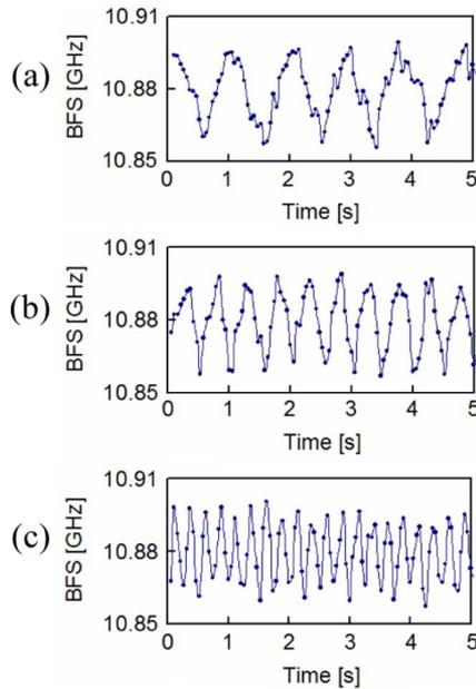
Fig. 4. Results of dynamic strain measurement with sinusoidal driving voltages applied to the PZT at (a) 1 Hz, (b) 2 Hz, and (c) 4 Hz, respectively. Note that the sampling rate is 19 Hz.
