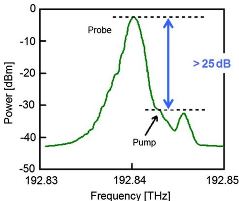
Fig. 2. (Color online) Measured optical spectrum of the SSBM output when the frequency of the MG was set to 2.83 GHz.
