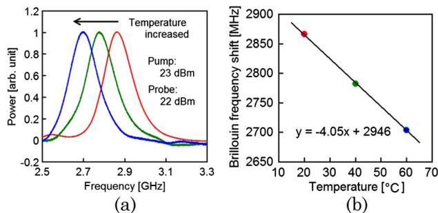
Fig. 5. (Color online) Dependence of (a) BGS and (b) BFS on temperature in POF.
