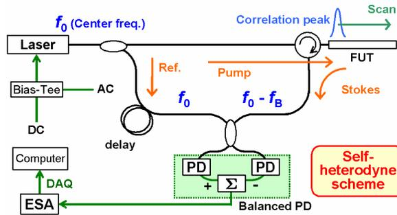
Fig. 1. Conceptual schematic of BOCDR system.
