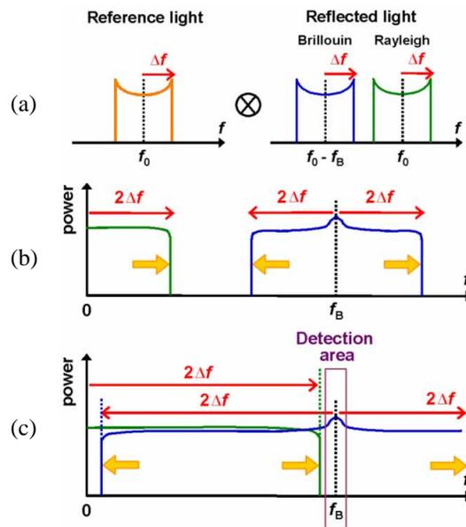
Fig. 6. Schematics of (a) optical spectra of the reference light and the reflected light when the frequency of the light source is modulated with the amplitude  $\Delta f$ , (b) electrical spectra with sufficiently small  $\Delta f$ , and (c) electrical spectra with large  $\Delta f$ .
