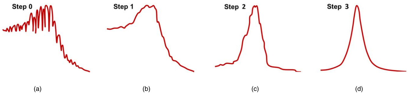
Fig. 1. (Color online) Schematic calculation procedures of the new method for detecting the Bragg wavelength. (a) FBG-reflected spectrum measured with a high resolution (step 0). (b) Spectrum intentionally measured with an extremely low resolution (step 1; optional). (c) Spectrum with the noise floor subtracted (step 2). (d) Lorentzian-fitted spectrum, from which the Bragg wavelength is derived (step 3).
