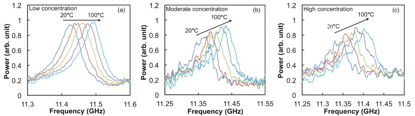
FIG. 1. Measured BGS dependences on temperature in EDFs with erbium concentrations of (a) 0.72 wtppm (low), (b) 1.20 wtppm (moderate), and (c) 2.28 wtppm (high).
