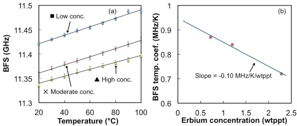
FIG. 3. (a) Temperature dependences of BFS in EDFs with different erbium concentrations. (b) Temperature coefficient of BFS in EDFs as a function of erbium concentration.
