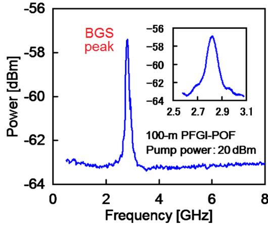
FIG. 2. (Color online) Measured BGS in the PFGI-POF at the pump power of 20 dBm. The inset shows the magnified view around the BGS peak.
