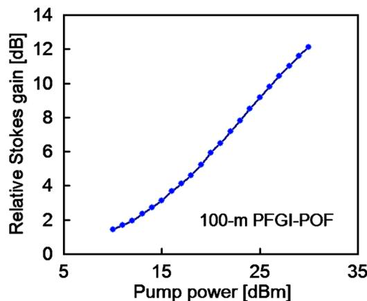
FIG. 3. (Color online) Relative gain of the Stokes light backscattered from 100 m PFGI-POF as a function of pump power.
