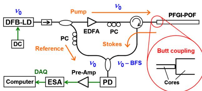
FIG. 1. (Color online) Experimental setup for observing Brillouin scattering in the PFGI-POF: DAQ, data acquisition; dc, direct current; DFB-LD, distributed-feedback laser diode; EDFA, erbium-doped fiber amplifier; ESA, electrical spectrum analyzer; PC, polarization controller; and PD, photodetector.
