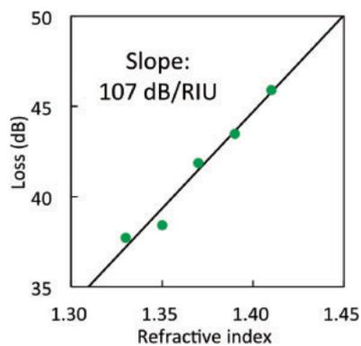
**Fig. 5.** Optical loss at the taper (excluding the initially induced loss) as a function of the refractive index of liquids. The measured data are shown as green circles, and the black line shows a linear fit.
