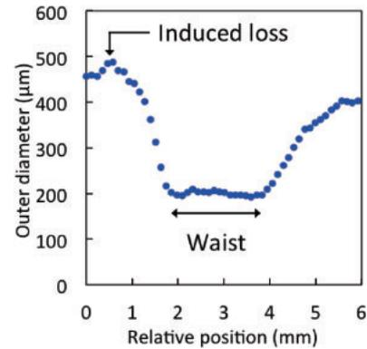
**Fig. 4.** Outer diameter distribution around the waist of the PFGI-POF taper.
