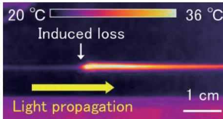
**Fig. 2.** Thermograph around the loss-induced point in the PFGI-POF.
