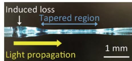
**Fig. 3.** Micrograph of the tapered PFGI-POF.
