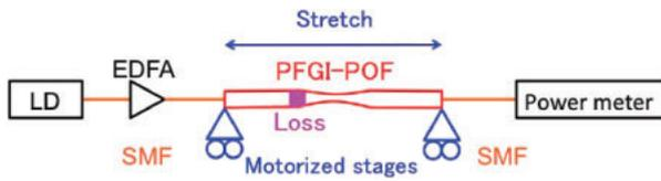
**Fig. 1.** Schematic of the experimental setup for PFGI-POF tapering. EDFA, erbium-doped fiber amplifier; LD, laser diode; PFGI-POF, perfluorinated graded-index polymer optical fiber; SMF, single-mode fiber.
